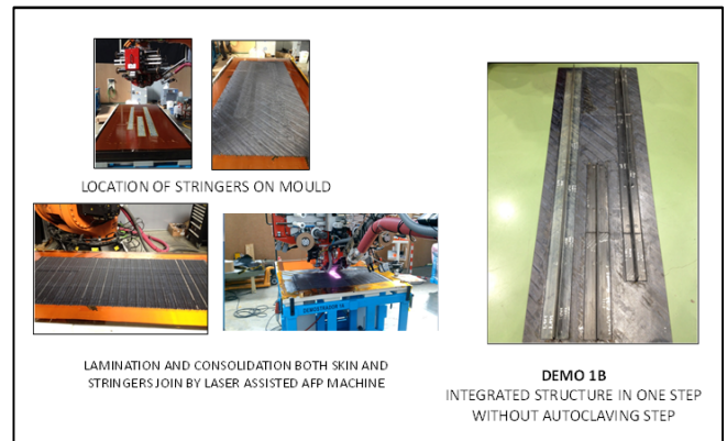
Figure 8. Feasibility demo of full stiffened wing panel with new concept of 8-tows machine.
