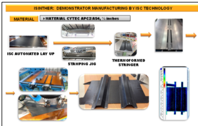
Figure 6. Co-consolidated full stiffened structure process.
