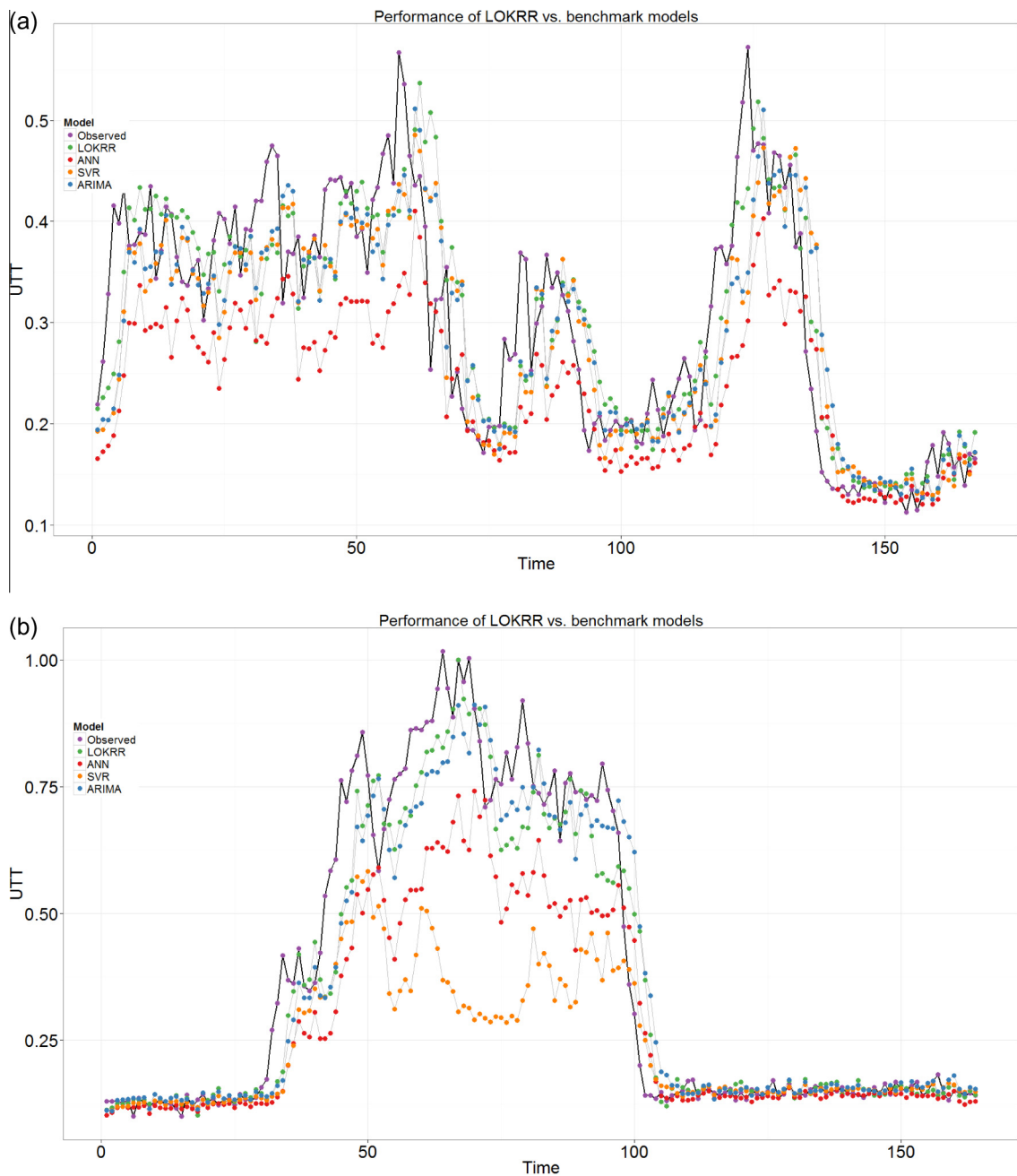
Fig. 10. Comparison of LOKRR with benchmark models at the 15 min interval on link 442, (a) on a typical weekday and; (b) during a non-recurrent congestion event.
