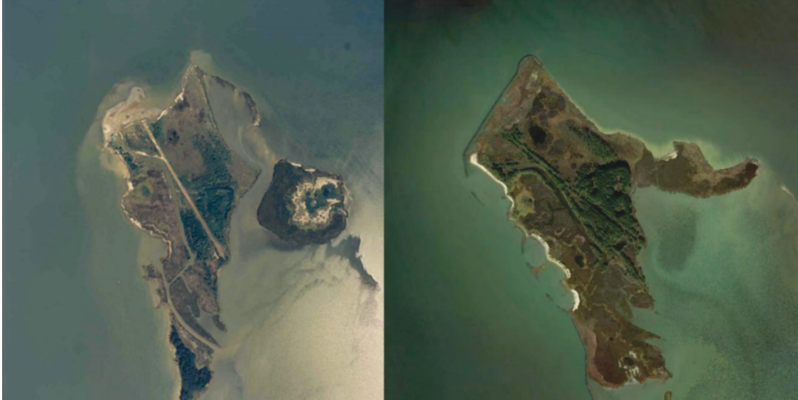
Figure 4. Barren Island before (left) and after (right) construction of breakwaters and restored marsh habitat (Images sourced from Google, DigitalGlobe 2017).
