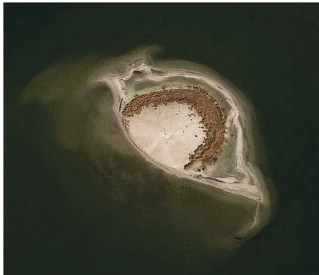
Figure 10. Mark-12 island and surrounding mudflat created using unconfined open water placement of dredge material two years post construction (2017 images sourced from Google, DigitalGlobe 2017).
