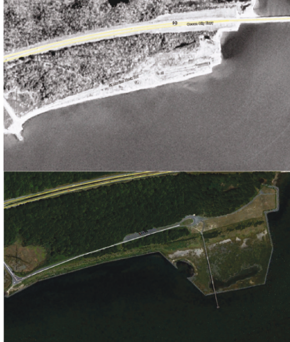
Figure 1. Isle of Wight before dredged material placement. Top: historic 1989 aerial image. Bottom: after dredge material placement and marsh establishment 2017 aerial image. (Images sourced from Google, DigitalGlobe 2017).
