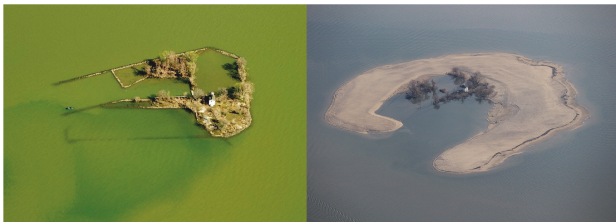
Figure 7. Battery Island before (left; 2011) and after (right; 2013) unconfined placement of dredge material.
