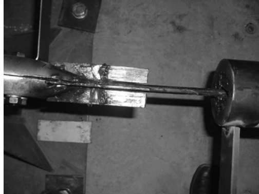
Figure 85. Pulled out core for dissipator D1
