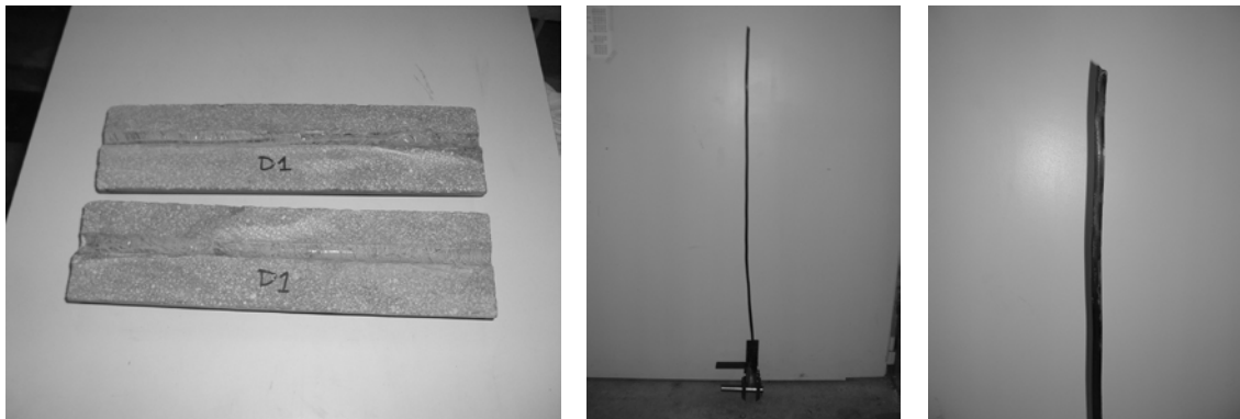
Figure 86. Mortar and core of dissipator D1
