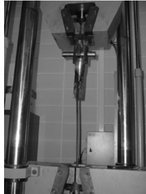
Figure 87. Pull-out test of connectors with adhesive only for dissipator D1
