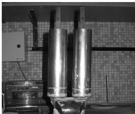
Figure 7. Two (short) dissipators prior to mortar pouring
