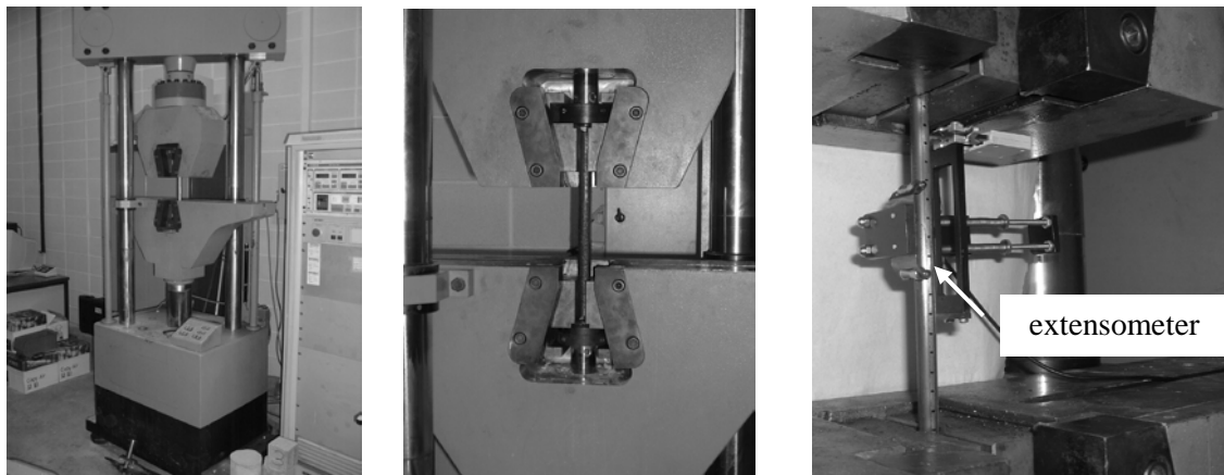
Figure 50. Testing of the steel core
