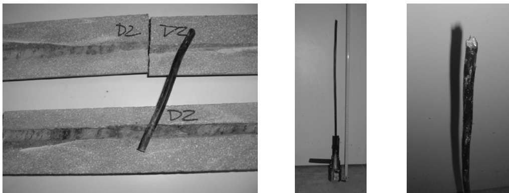
Figure 113. Mortar and core of dissipator D2
