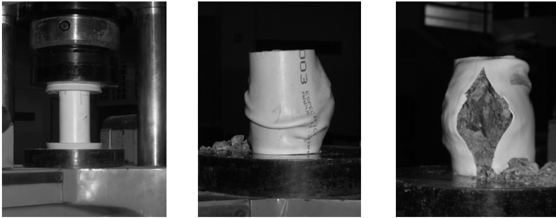
Figure 19. Testing of grout and mortar specimens coated with PVC
