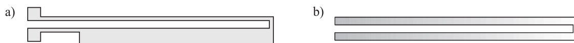
Figure 1: a) Classic shape of MEMS actuator, b) New shape of FGM actuator
