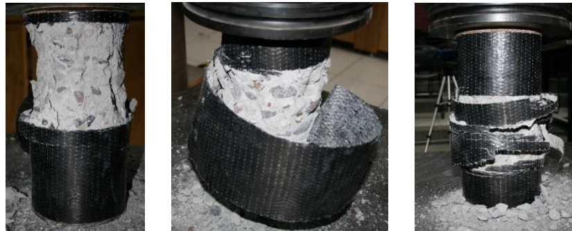
Figure 2. FRP specimens after compression test.
