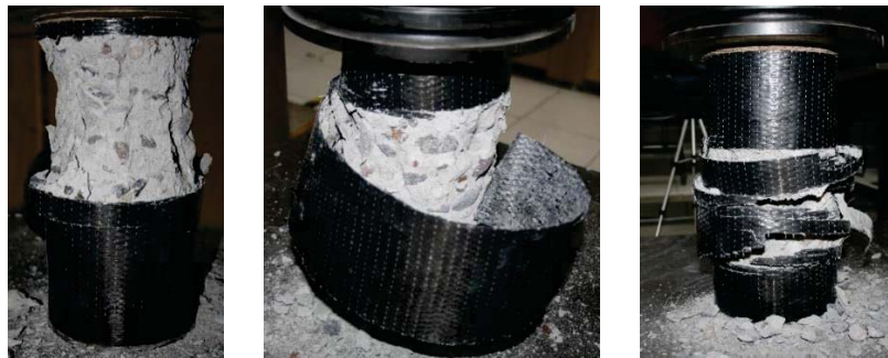
Figure 2. FRP specimens after compression test.
