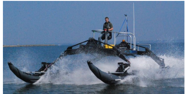
Fig. 1 Spray generated by the WAM-V hull at 21 knots [25]. Courtesy of Prof. Mehdi Ahmadian, VirginiaTech, USA
