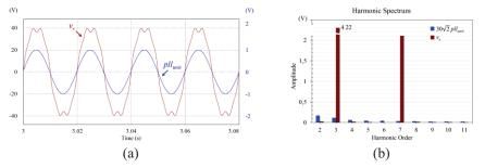
**Fig. 5.** Simulations of the PLL algorithm: (a) Power grid voltage ( $v_s$ ) and output signal of the PLL (*pllunit*); (b) Detail of the harmonic spectrum of the power grid voltage ( $v_s$ ) and output signal of the PLL (*pllunit*).
