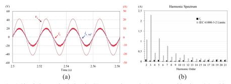
**Fig. 6.** Simulation results during the G2V operation mode: (a) Power grid voltage ( $v_s$ ), grid current ( $i_s$ ), and grid current reference ( $i_s\_ref$ ); (b) Detail of the harmonic spectrum of the grid current ( $i_s$ ) in comparison with the limits established by the standard IEC 61000-3-2.
