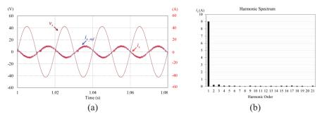
**Fig. 8.** Simulation results during the V2G operation mode: (a) Power grid voltage ( $v_s$ ), grid current ( $i_s$ ) and grid current reference ( $i_s$  ref); (b) Harmonic spectrum of the grid current ( $i_s$ ).
