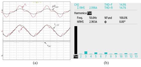
**Fig. 11.** Experimental results during the G2V operation mode: (a) Power grid voltage ( $v_s$ : 20 V/div), PLL output signal (*pllunit*: 1 V/div), grid current (*is*: 2 A/div), grid current reference (*is\_ref*: 2 A/div), DC-bus voltage ( $V_{DC}$ : 20 V/div) (Time: 5 ms/div); (b) Harmonic spectrum of the grid current (*is*).
