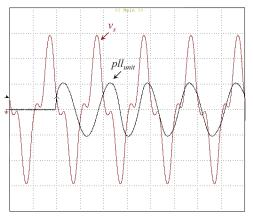
**Fig. 10.** Experimental results of the power grid voltage ( $v_s$ : 20 V/div) and the output signal of the PLL algorithm (*pll*<sub>unit</sub>: 1 V/div) (Time: 10 ms/div).
