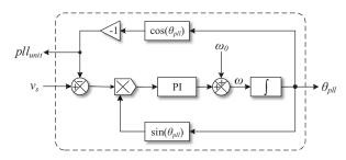
Fig. 4. Phase-locked loop algorithm used to synchronize the slow EV battery charger with the power grid voltage.
