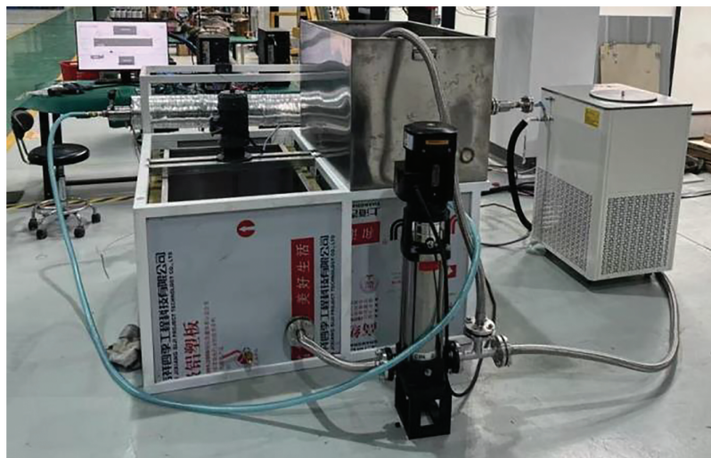
Figure 3: Miniaturized drilling fluid heat exchange cooling device physical diagram
