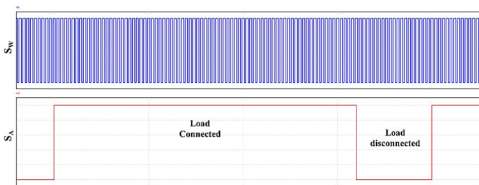
Figure 5: Switching pattern of the main switch ( S_w ) and the load switch ( S_A )
