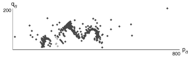
Figure 13. Frictionless compaction of the flanged component with the elliptic model. Final distribution of Cauchy stresses at Gauss-point level on the meridian plane q_{\bar{\sigma}}-p_{\bar{\sigma}} . Dark diamonds indicate plastic steps and light diamonds indicate elastic steps.
