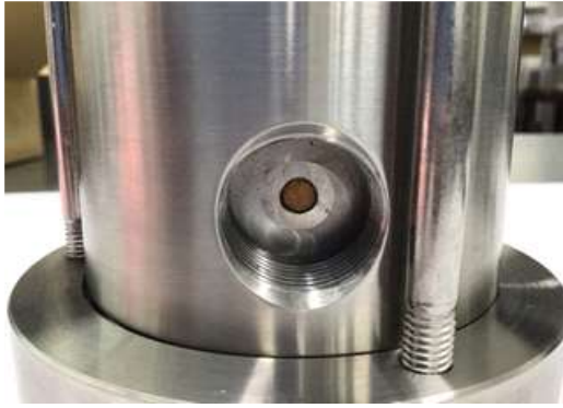
Figure 4. Position for installing of pressor sensor.
