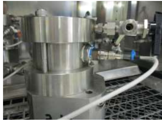
Figure 6. Connected steel mould with pressure sensor.
