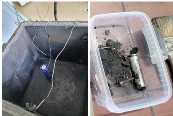
Figure 2: State of the battery sample before (left side) and after the experiment (right side)
