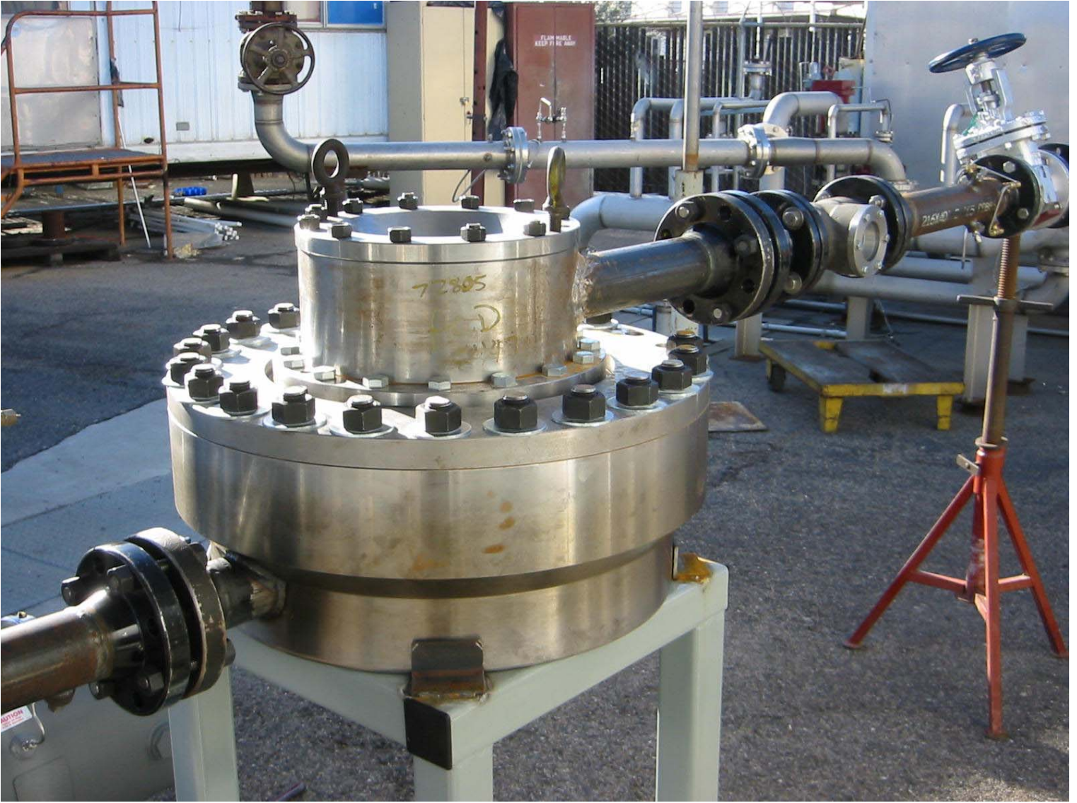
Figure 44 Integral Separator During Testing
