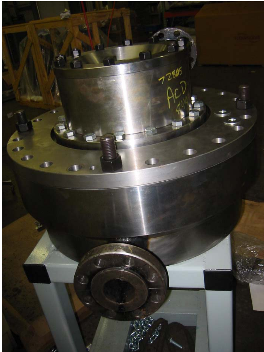
Figure 34 Integral Separator Assembly Showing Nozzle Inlet
