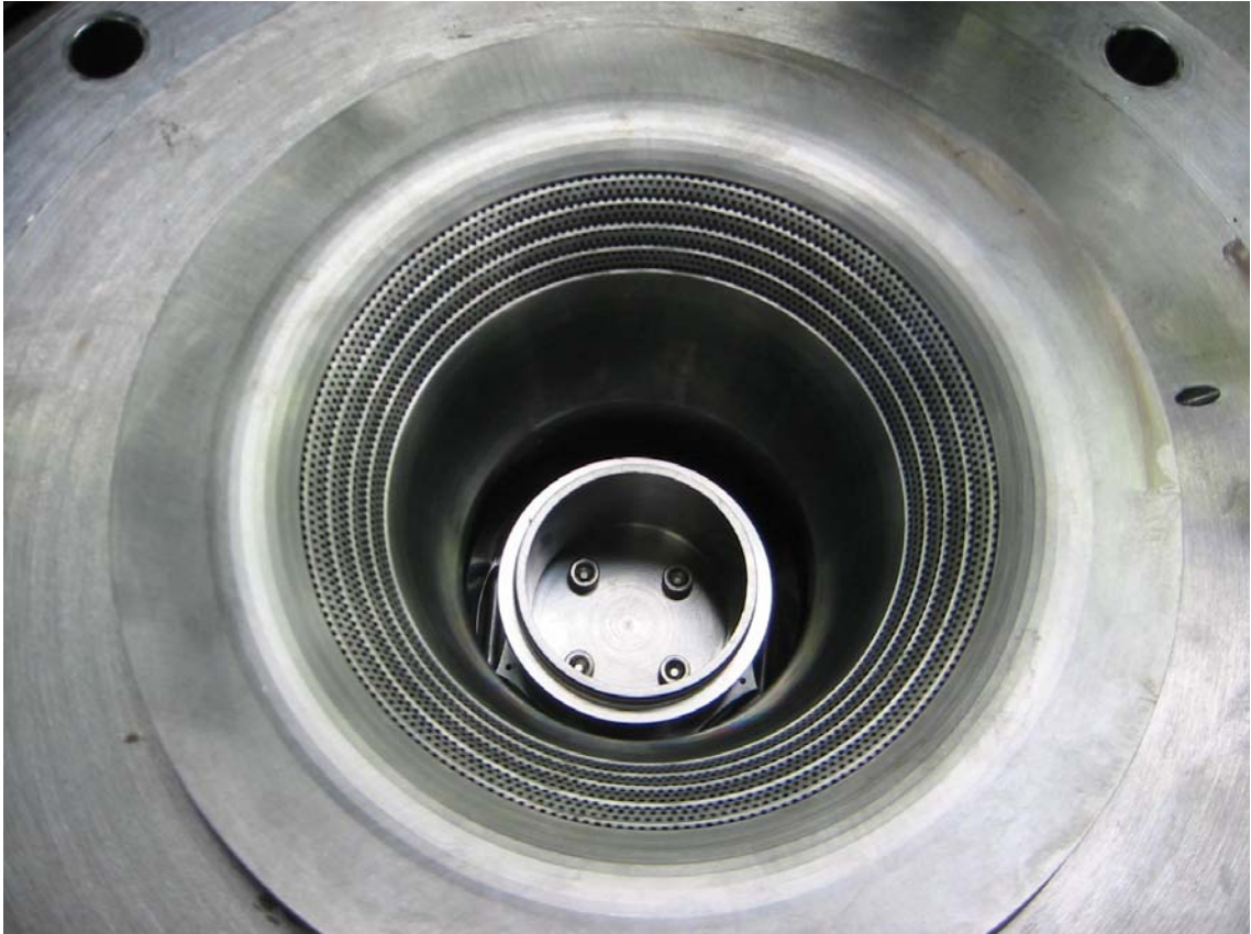
Figure 32 Interior of Vortex Chamber and Diffuser Outer Wall
