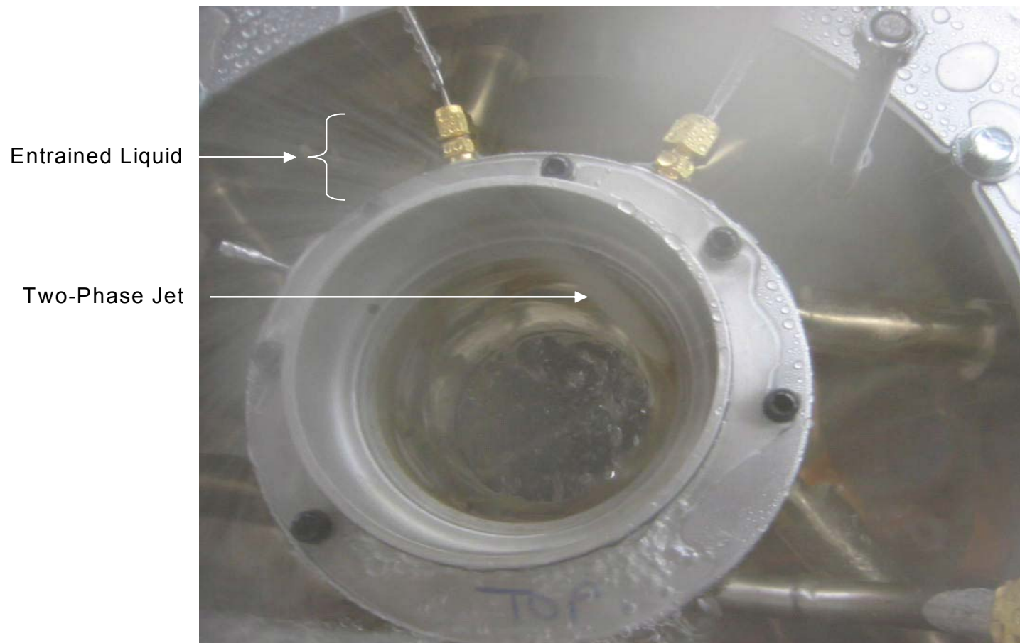
Figure 51 Operation with Mal-Distribution of Liquid, Top Removed
