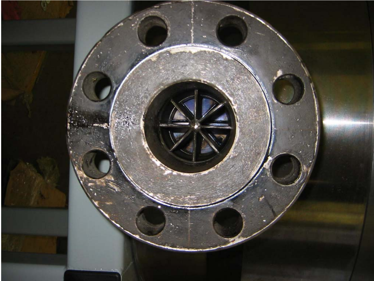
Figure 33 Inlet Flow Splitter
