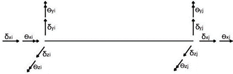
Figure 2: Degrees of freedom in 3D elements
