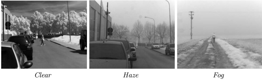
Fig. 5. Images acquired in the SWIR spectrum ( 1.0 - 1.7 \mu m ) –filter F2 – with different visibility conditions during summer, autumn and winter respectively
