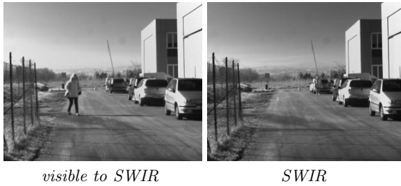
Fig. 9. Images acquired in the whole visible to SWIR ( 0.4\text{--}1.7\ \mu\text{m} ) spectrum –filter C – and in the SWIR only ( 1.3\text{--}1.7\ \mu\text{m} ) spectrum –filter F1 – respectively: almost invisible in the first image, the background mountains become quite clear in the second image
