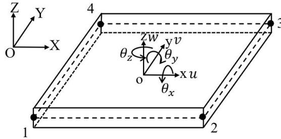
Figure 1 Four-node quadrilateral inverse-shell element iQS4
