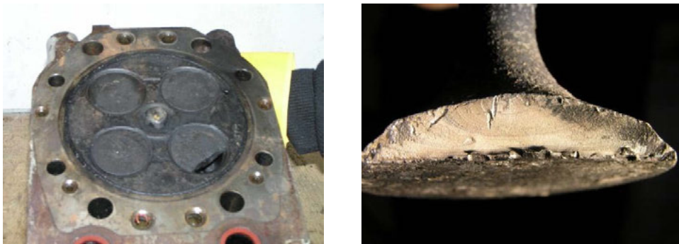
Figure 1. Cylinder head of submarine diesel engine type MB820 with broken exhaust valve
