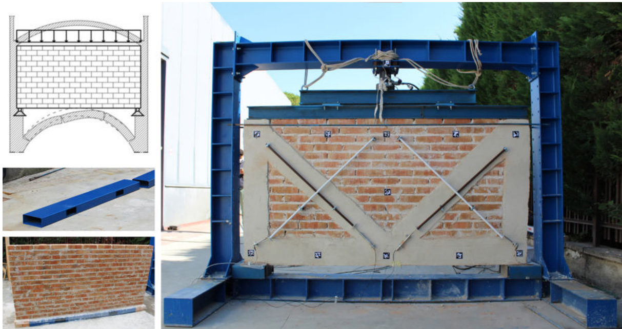
Figure 1: Starting from the top row: example of an “in falso” wall triggering progressive collapse phenomena. Pics of the elements characterizing the setup, in order temporary steel support and construction on it of one of the prototypes. On the right, beginning of the test with the wall already instrumented (Test 3).
