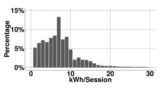
Figure 5. Distribution of kWh charged at level 2 charging stations.
