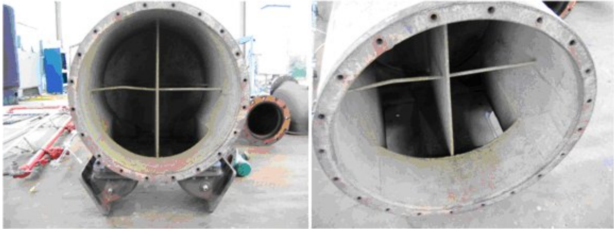
Figure 5-24. Photographs of Internal Geometry of Exhaust Manifold
