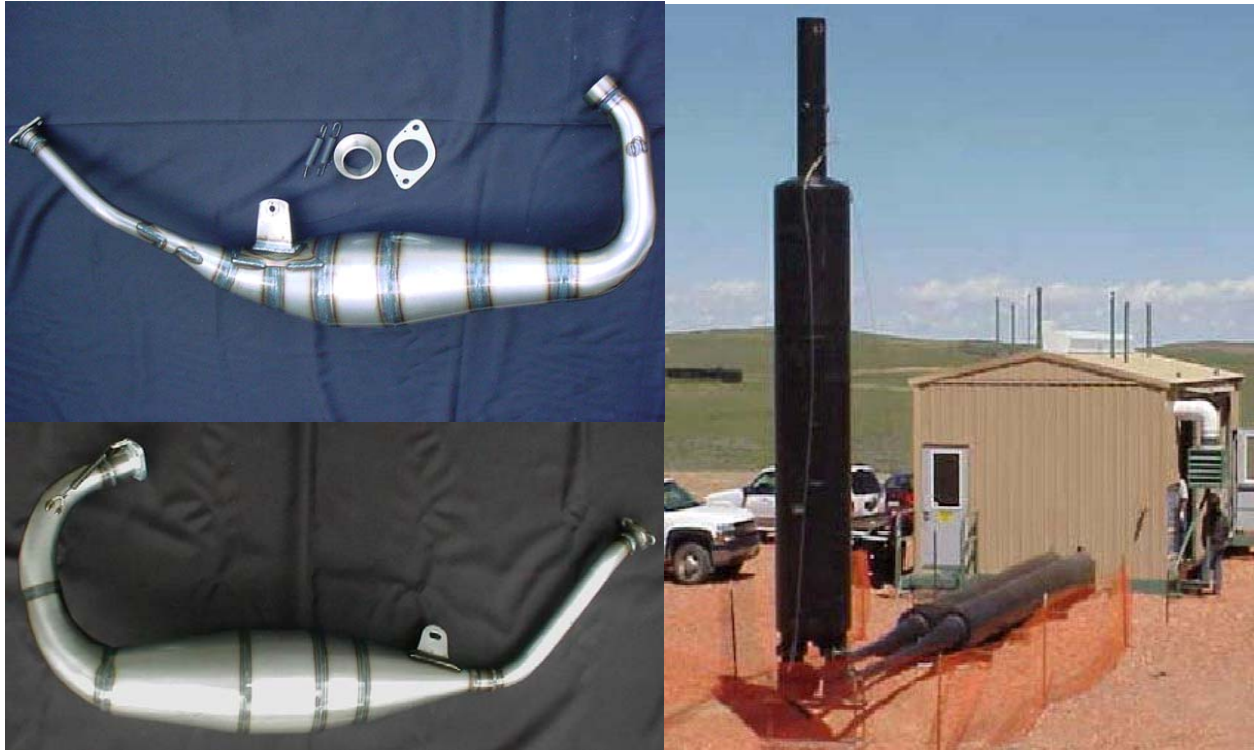
Figure 6-2. Photographs of Expansion Chambers (Motorcycle Application at Left & AJAX™ Application on Right [4] )
