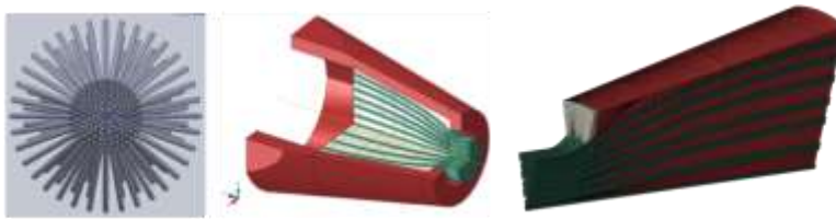
Figure 3: FE model included conical socket housing, cast zinc, and individual wires.
