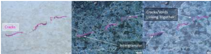
Figure 9: Intergranular cracks present adjacent to cable/zinc slug boundary as seen in brightfield, dark field, and cross-polarized illumination. Klemm's 1 Reagent tint etch at 500X magnification.
