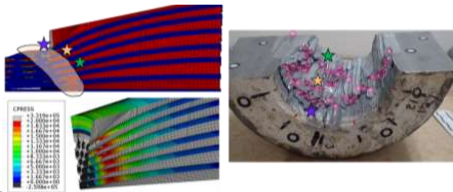
Figure 8: Highest stresses were not predicted to be planar; failure surface followed a spheroid shape, matching stepped patterns seen in forensic evidence.
