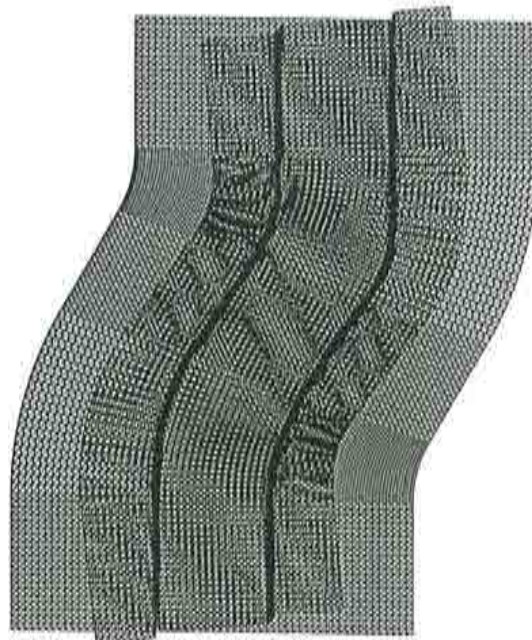
Figure 5.31 Deformed mesh after the stamping stage superimposed on the original mesh.
