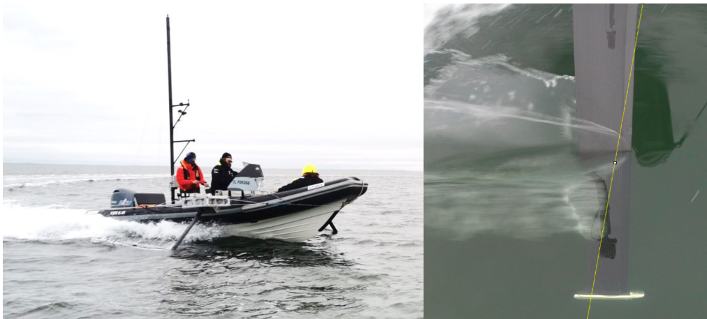
Left - test set up on the semi-rigid motor boat equipped by two kitefoil shafts. Right - Ventilation observed on a kitefoil shaft during the test
