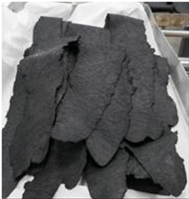
Figure 5. Samples after extrusion process – powder gel coat laminated.
