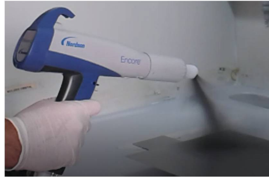
Figure 6. Powder gel coat applied in a metallic plate.
