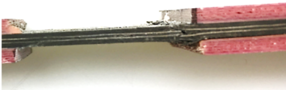
Figure 12. Autoclave curing process – compression test failure example.
