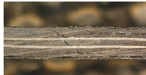
Figure 14. Autoclave curing process – ILSS test failure example.
