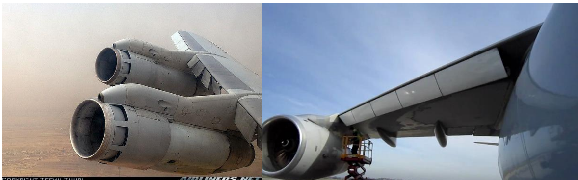
Figure 3: (left) sealed Krueger flap at the Boeing B707 operated sequentially (image obtained from airliners.net © Teemu Tuuri); (right) inboard Krueger flap at the Boeing B747 operated in groups (image obtained from youtube.com © user/Jet3TV)
