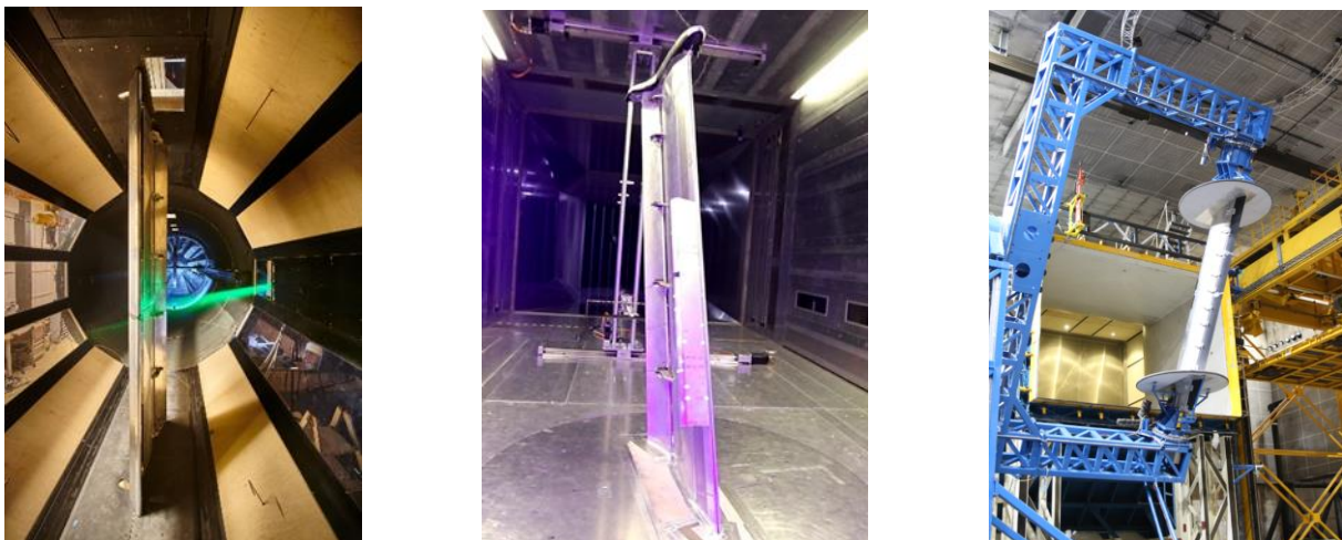
Figure 6: wind tunnel model installations used in the UHURA Project: (left) DLR-F15-LLE mounted wall-to-wall in ONERA L1; (middle) DLR-F15-LLE mounted as swept cantilever wing in DNW-NWB; (right) DLR-F15LS-LLE mounted as swept wing in the open test section of DNW-LLF
