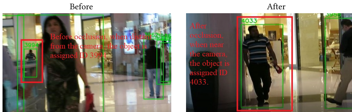
Figure 6: Failure case: the target is initially small and far from the camera, then after prolonged full occlusion reappears near the camera with a different assigned ID
