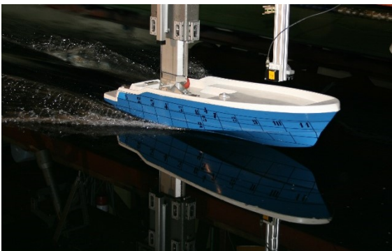
Figure 11a. Experimental dynamic wetted surface and wetted length at Fr = 1.96 .
