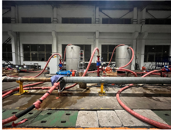
Figure 5: Layout of hydraulic lift type dual-gradient drilling indoor physical simulation experiment system
