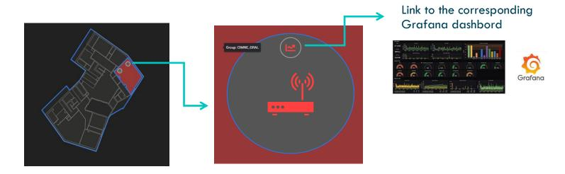
When an alert is triggered the platform detect in real time the geolocation of the group and device with problems.
