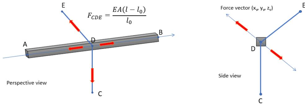
Figure 6: Sliding of a cable over a beam-element
