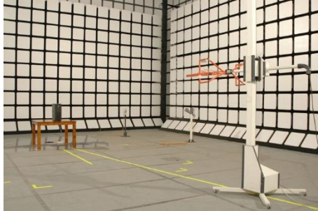
Figure 3: The anechoic chamber used for the EMSE tests.
