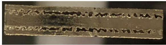
Figure 7: Metallization of the hybrid (Carbon/flax composite)
