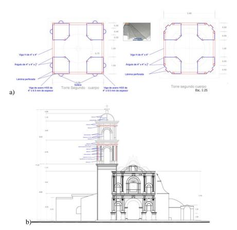
Figure 8: Reconstruction of the belfry with perforated steel plates: a) plan view; b) frontal view
