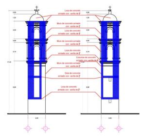
Figure 7: Reinforcement of a bell tower with concrete walls
