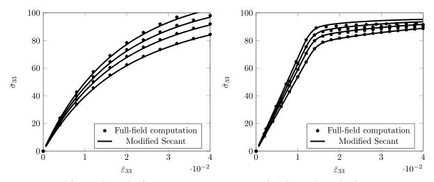
a. Linear elastoplastic case b. Elasto-viscoplastic case Figure 1. Macroscopic stress evolution with the prescribed macroscopic strain as predicted by the modified secant model and the full-field calculations as a function of defective inclusions. Material data are respectively given in table 1 and 2.
