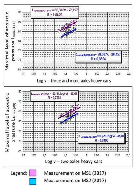
Fig. 3: Regression lines of the maximum levels of acoustic pressure from the decimal speed logarithm for vehicle categories 1, 2a, and 2b on measurement sections MS1 and MS2 evaluated from measurements on 14 September 2017.
