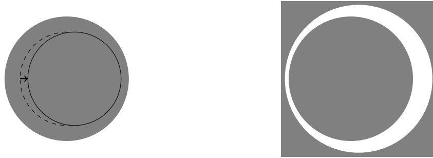
(a) The two circular metal patches can show some misalignment resulting in degradation of antenna performance. (b) The circular antenna patches can drift towards the fuselage panel which can lead to unwanted electrical coupling between the patch and the fuselage panel.
