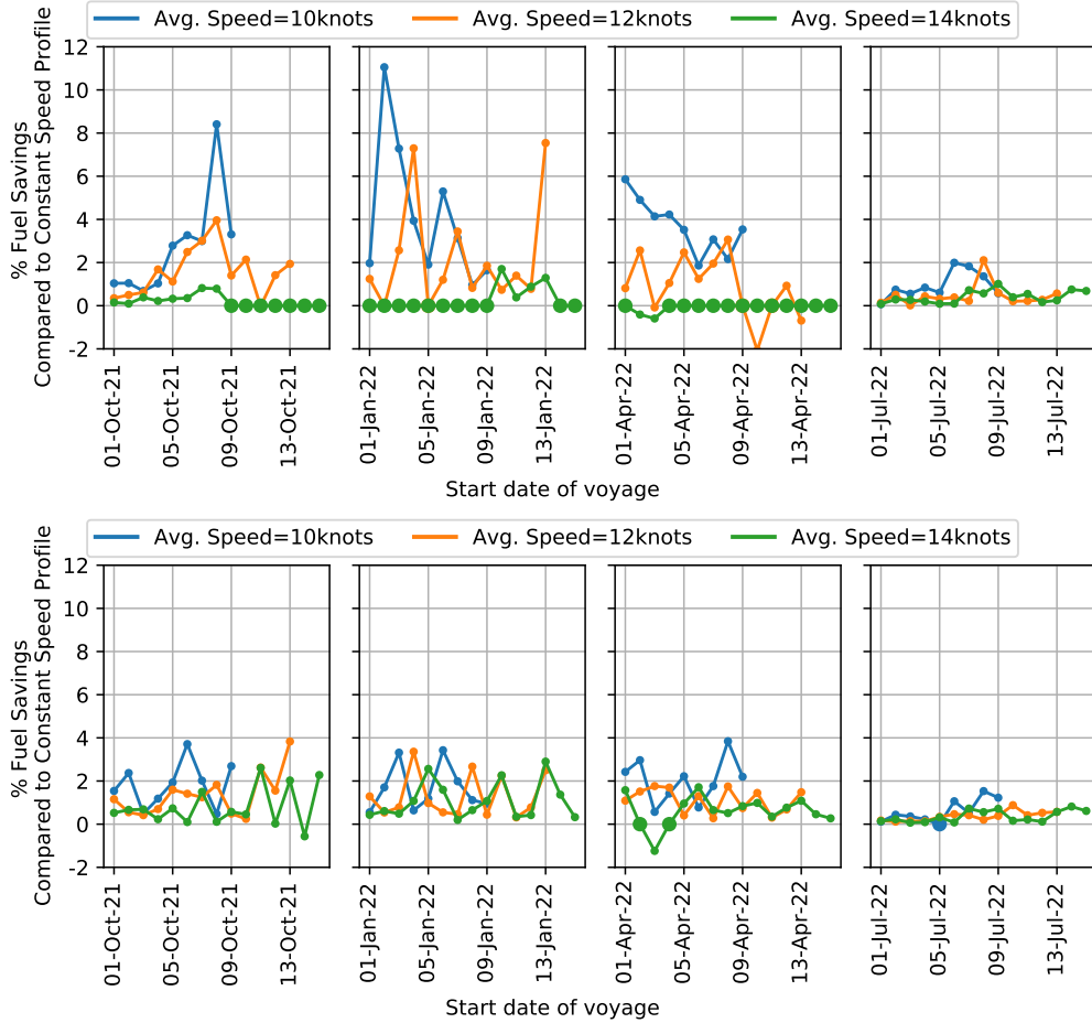
Figure 3: Fuel savings on westbound (top) and eastbound (bottom) voyages at different average speed and seasons for Capesize bulk carrier.
