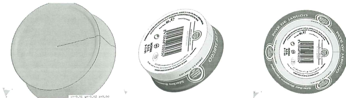
Fig. 4: Can stamping simulation made by Quanteck ATZ for Metalpack SA: after deforming the sheet mesh to the final can state, the decorative labels are applied to the mesh and then its original flat shape is restored to get the deformed images, ready for the press ( courtesy of Quanteck ATZ, Metalpack SA).
