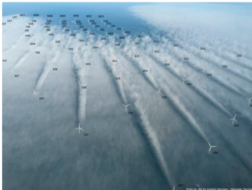
Figure 1: Wind turbine wake visualized by fog in Horns Rev Wind Farm [1]
