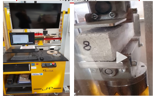
Figure 4. Scheme and images of 3-point Flexure Test unit
