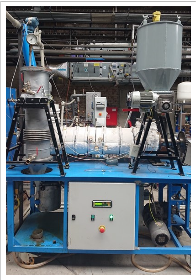
Figure 20. Installed small-scale pyrolysis unit.
