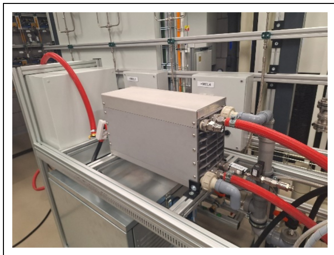
Figure 15. Installed Nedstack FCS 8-XXL fuel cell stacks as part of the system for hydrogen-to-electricity conversion.
