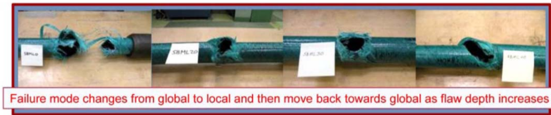
Figure 11 Failure Mode for Burst Tested Flawed FRP with Increased Flaw Depth
