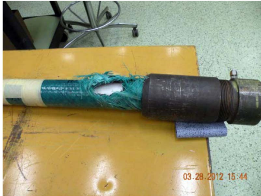
Figure 14 Burst Test of FRP Following 8000 Full Pressure Cycle Fatigue Test
