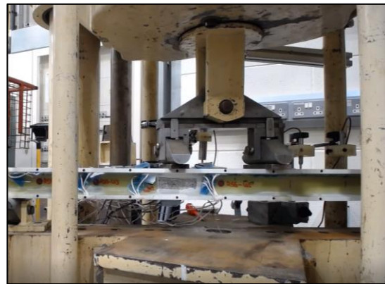
Figure 1: Four-point bending testing of the demonstrator.
