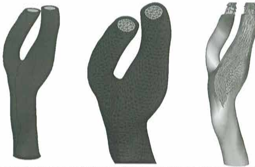
Figure 1: Modeling of blood flow in the bifurcation of carotid artery. Geometry (left), the element mesh (middle), and a snapshot of the simulation results (right). The colors of the artery surface and the vectors indicate the displacements of the artery and the velocity of the blood, respectively. The geometry is meshed in GiD and the results are computed and visualized with Elmer.
