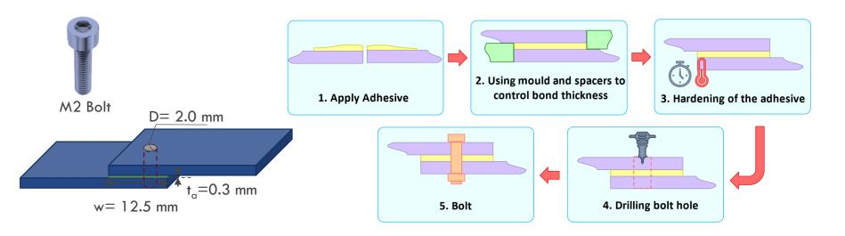
Applied Clamping Torque: 0.6-0.7 Nmm
