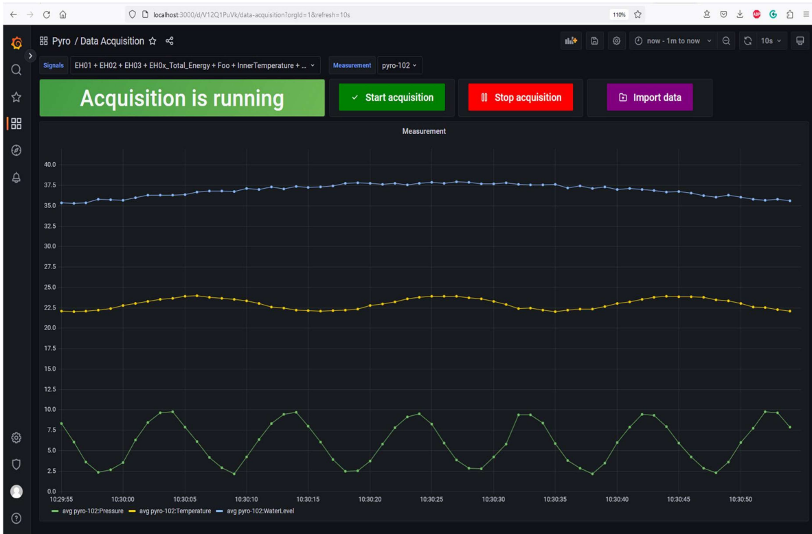
Figure 12. Data acquisition dashboard during active measurement of pyrolysis provided by ABB, green curve represents Pressure, yellow represents Temperature and blue represents Water Level.
