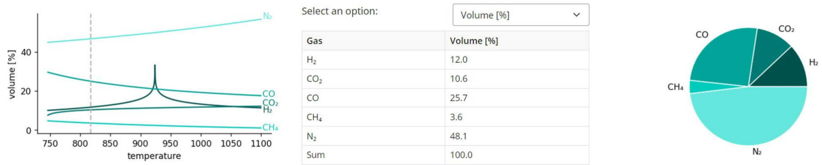
Figure 5. Composition of syngas; Select an option can be in Volume [%], Volume [m 3 ], mol, Mass [%], Mass [g], and Mass [kg].
