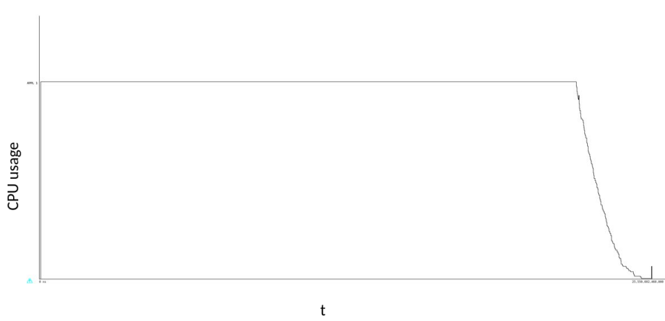
Figure 4.2: CPU usage of asynchronous Monte Carlo algorithm, running with PyCOMPSs with 41 worker nodes / 1968 CPUs. CPU usage is constant and equal to 100% of the machine during the whole runtime. The problem is the wind engineering two-dimensional benchmark (see [14] for details).
