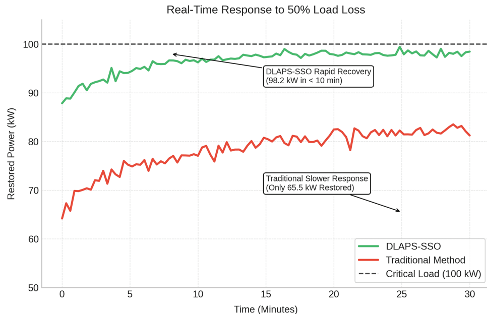
Figure 17: Real-time line graph for 50% load loss
